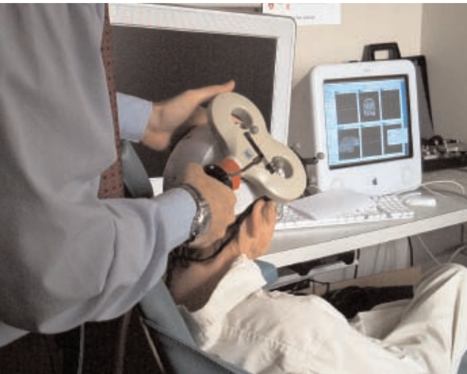
This image displays a picture of TMS being applied by an experimenter. Both the coil and the subject have affixed to them a tracking device so that the head/coil position can be monitored in real time. Therefore, the motor cortex can be accurately targeted and stimulated in patients with stroke to improve motor function. (Image courtesy of Dr. Felipe Fregni)
